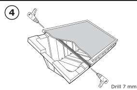
Use the profiles to drill 4 holes (7 mm) in the edges of the ConSole (please refer to diagram).
