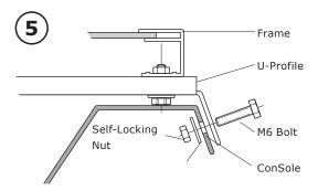
Mount the profiles onto the ConSole with the supplied mounting materials (please refer to drawing). Please make sure that the washer is placed between the nut and the ConSole.
